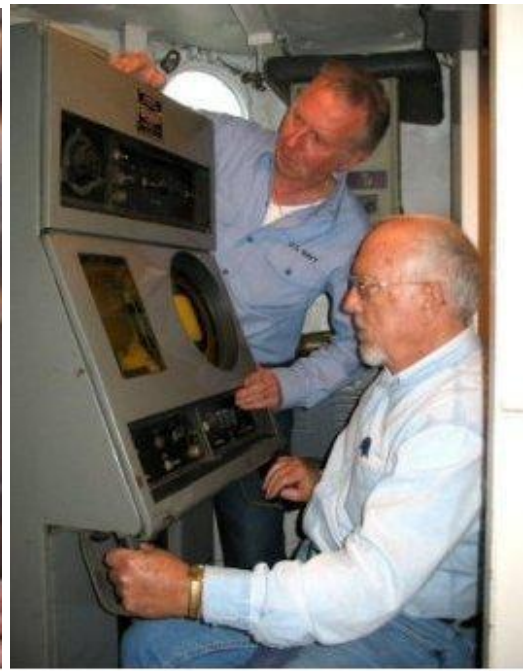
Sonarmen Ron Mazure on Bob Donlon check out the newly installed QJB sonar stack.
