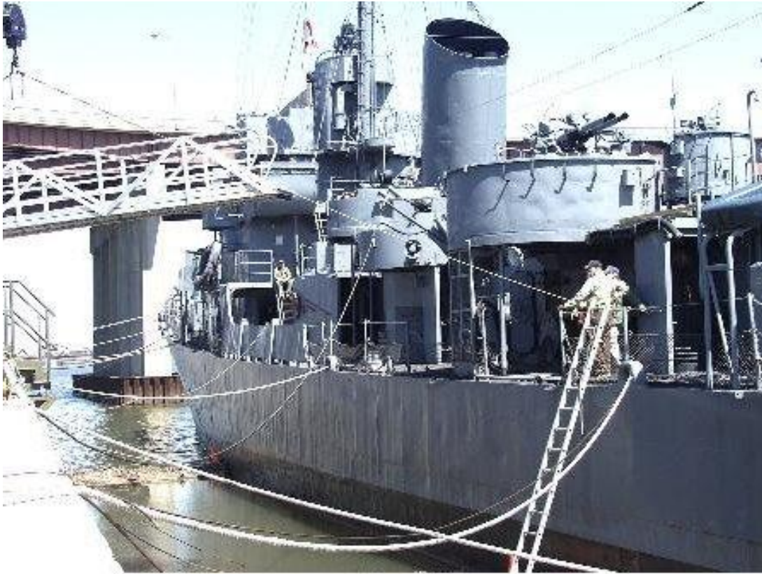
Rigging the brow on the Albany side.
