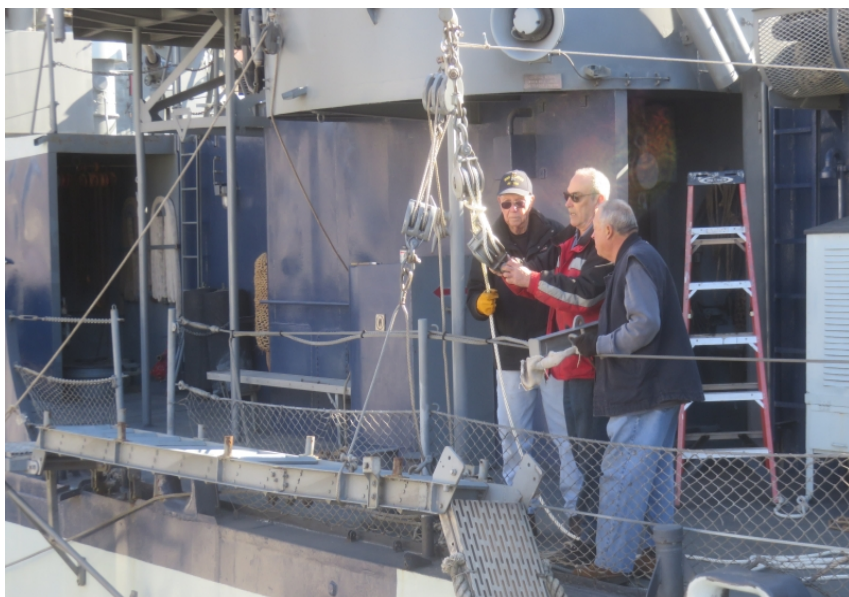
The deck gang lowered the accommodation ladder for the season.
