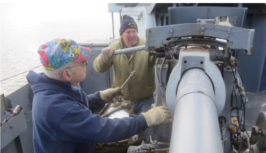
Doug Tanner and Danny Statile did the final disassembly of the gun 31 sightsetter.
