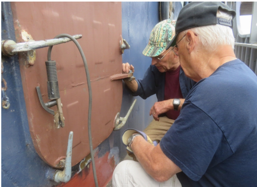
Checking the fit on the deck gear locker door.
