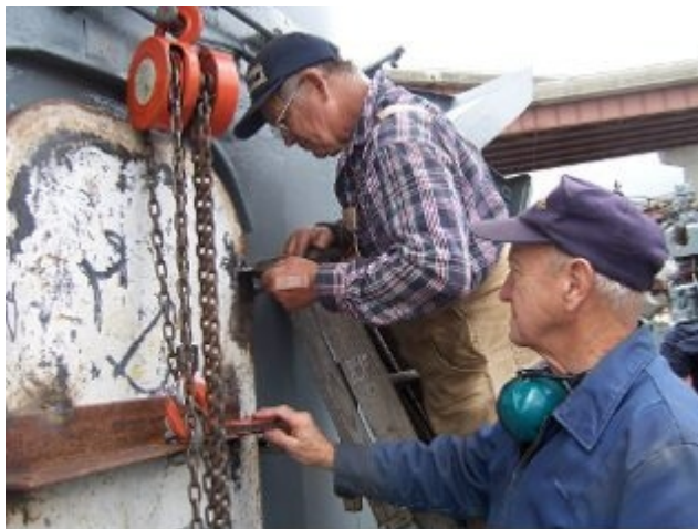
Laird Confer and Roy Brandon fitting the watertight door just aft of the hedgehog.
