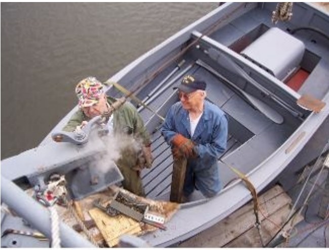
Doug Tanner and Super Dave work to disassemble the forward davit head block
