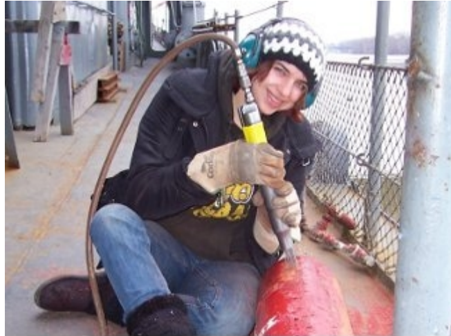
New volunteer Alexandra Scavelli scaling B-3 CO2 cylinders.
