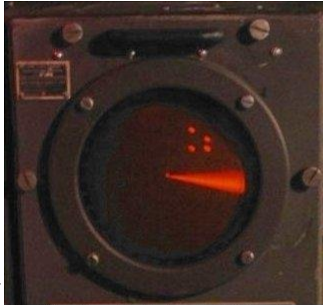
The SA radar with its simulated display. Looks like four ships at 045 degrees.
