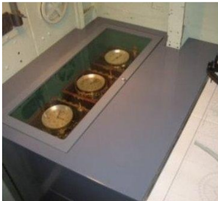
Tom Moore built a new table for the chartroom in which Erik Collin installed a chronometer well.
