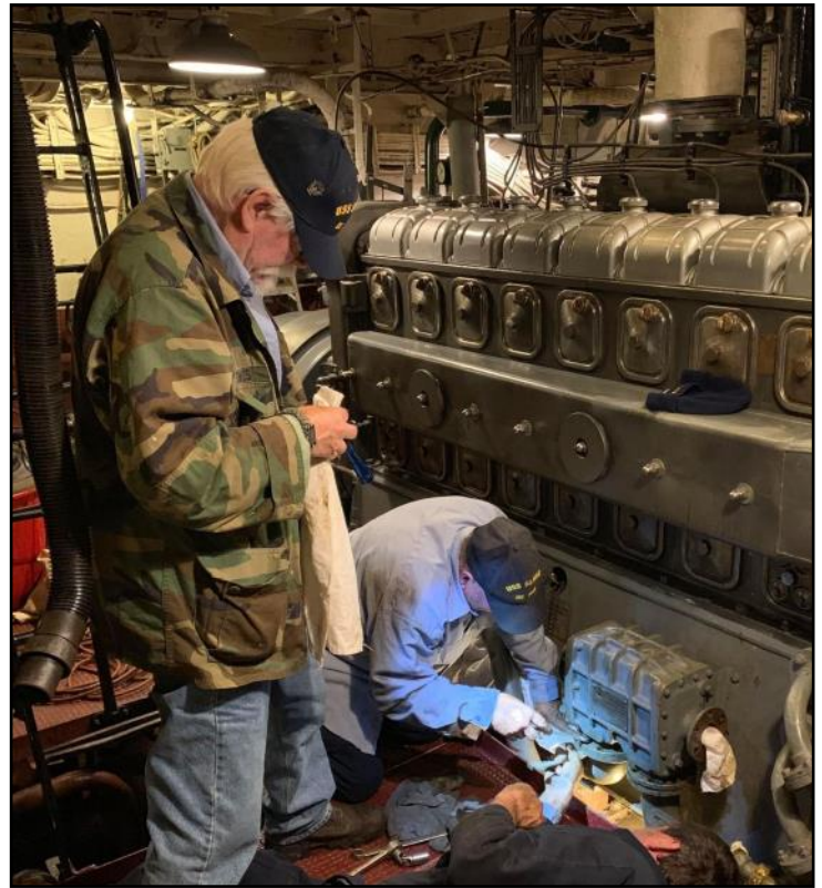
The engineers are removing an oil cooler.
