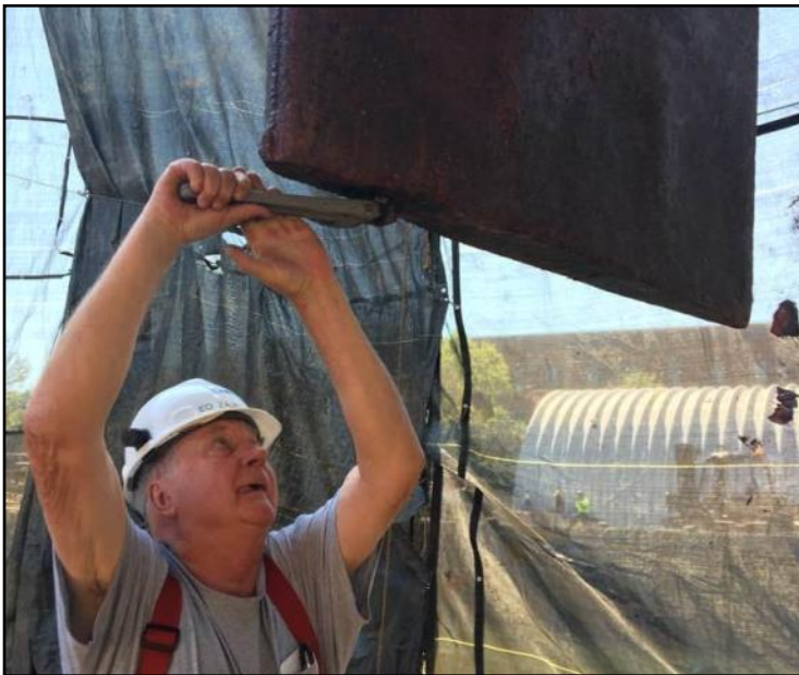
Ed checks the rudders for leakage.
