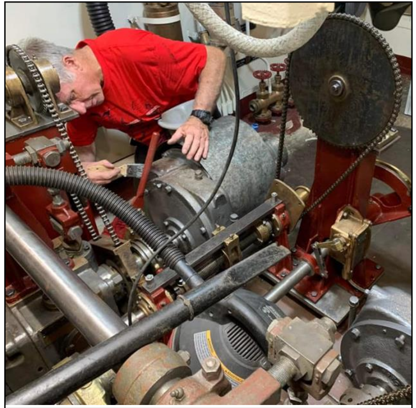
Gary Sheedy continues his work restoring the after steering compartment.
